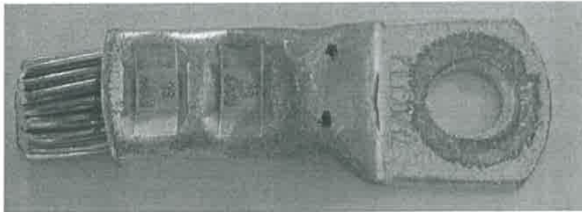
Figure 1: Tested cable lug.
