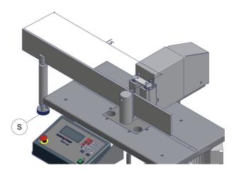
Use the support arm (S) for shank lengths "Is" of 1m to 2m.
