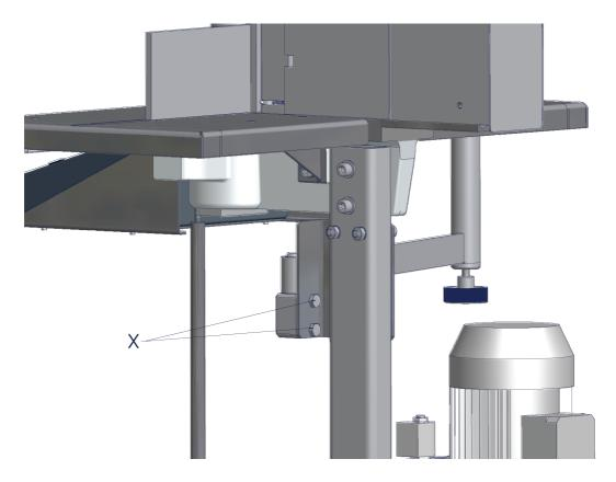
Fix the support arm to the bracket using 2 bolts (X).
