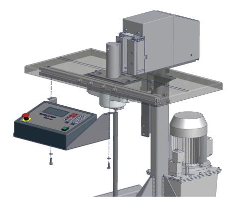
3. Screw the control unit onto the bending table loosely.
